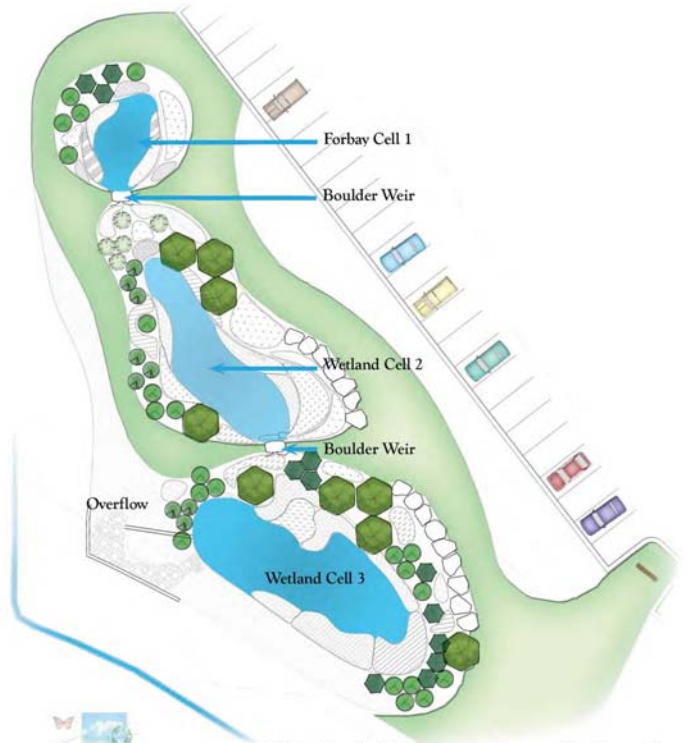
Bethel Elementary School Constructed Wetland
